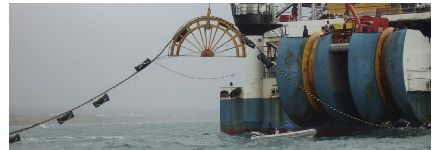
Export Cable Laying Vessel
